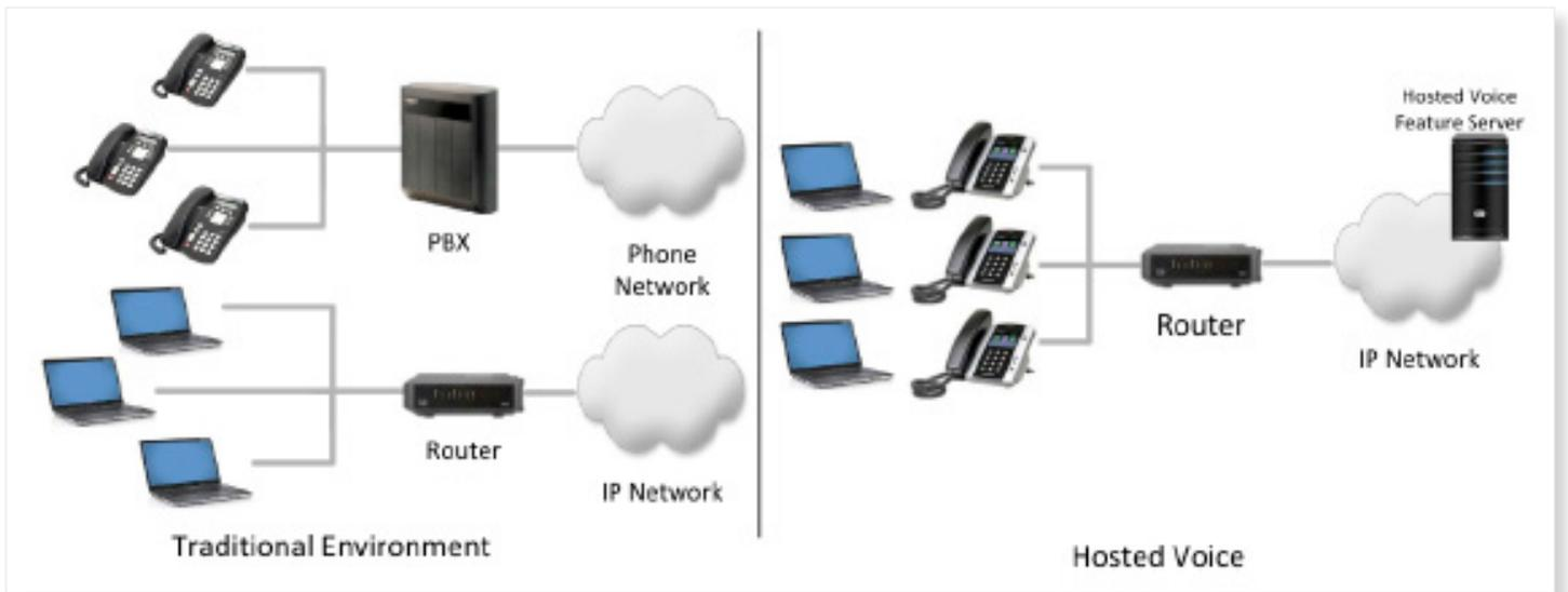
***In a traditional environment, multiple connections are required to deliver voice and data, and multiple pieces of equipment are needed. With Hosted Voice, a single IP connection delivers everything you need for voice and data, including the phone system functionality.***
